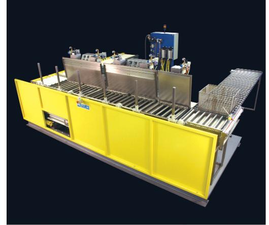
RAMCO manufactures two automation systems depending upon the requirements of the process—RamTough and RamNet. Both systems feature our **patented multi-arm walking beam** with simultaneous transfer of all baskets for maximum productivity. Each system is built on a heavy duty I beam fabricated base for accuracy, stability, and ease of shipping and installation.
